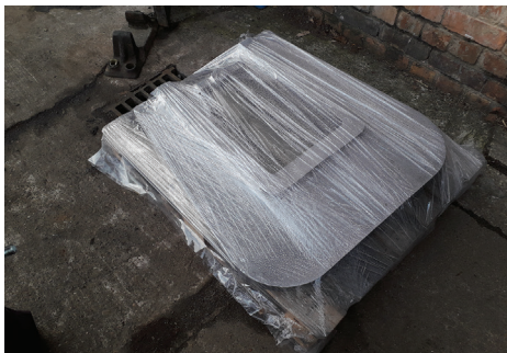
The first of the newly delivered horn guide castings wrapped in industrial cling film at Ruddington Locomotive Works in November 2018. MIKE FAIRBURN
