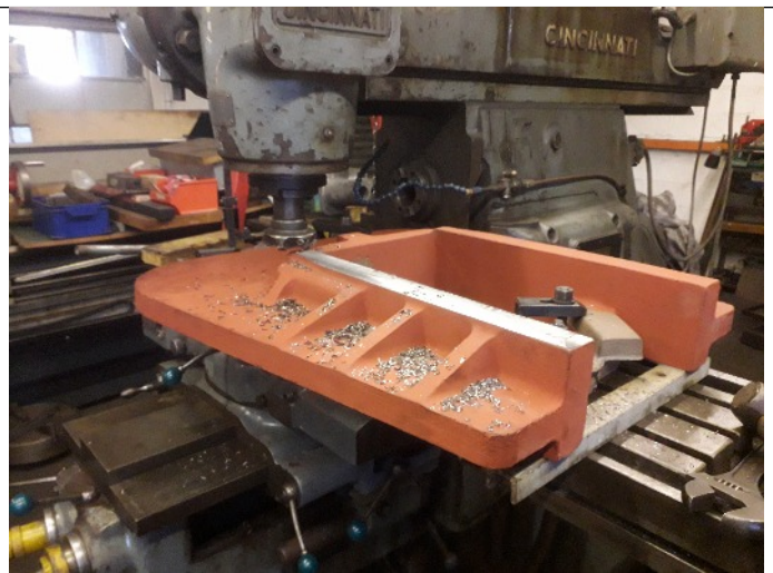
The first of the main frame hornblocks being proof machined at Ruddington at the beginning of February, 2019. MIKE FAIRBURN
