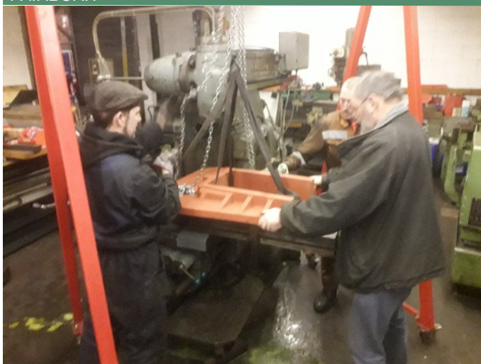
The lid of the oil pot on the Valve Spindle Guide being machined by Ken Harrison. KEN HARRISON
