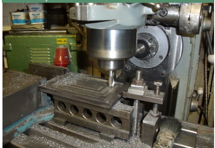
The lid of the oil pot on the Valve Spindle Guide being machined by Ken Harrison. KEN HARRISON
