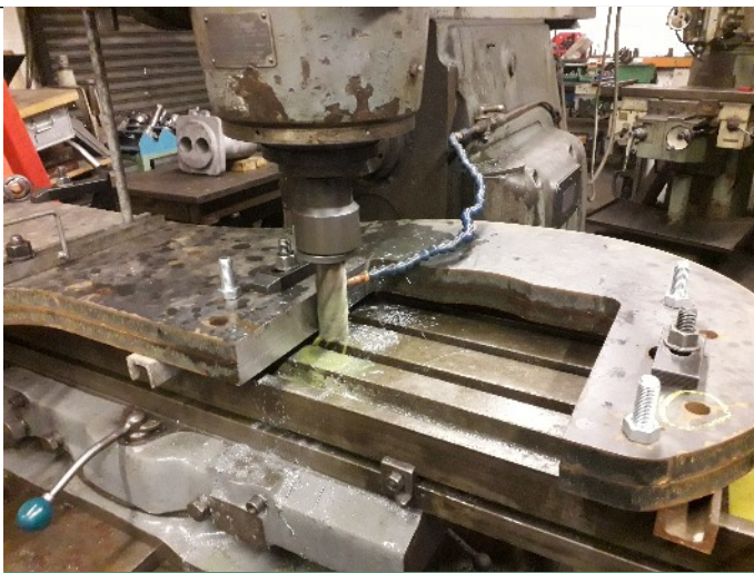
On 12 th January, 2019 the machining of the hornblock recesses is underway at the Ruddington Locomotive Works. MIKE FAIRBURN
