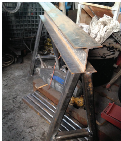
One of several trestles being built to support the erection of the frames. SIMON BURTON
