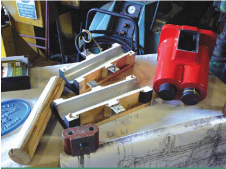
Ken Harrison's meticulous work on display at the Annual Supporters Day. The valve spindle guide pattern complete with its oil box is seen (painted red) together with the core patterns. The finished valve spindle guide will be bolted to the motion stretcher. DENNIS WILCOCK
