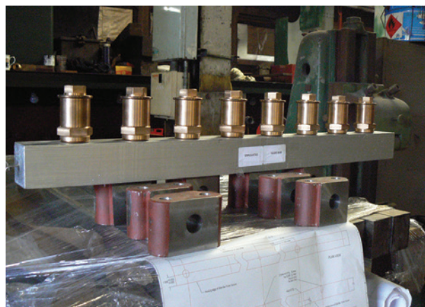
Seen on the Supporters Day the horizontal silver beam is a mock up of a slide bar. This is standing on the slide bar support blocks and below that are the actual slide bars that have now been fully ground. On top of the whole are the eight brass oil pots manufactured by Ken Harrison that will fit on to the slide bars. DENNIS WILCOCK
